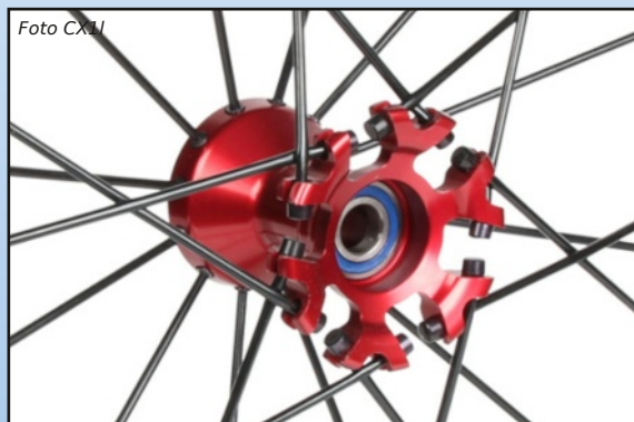
Spinergy CNC milled hub, 1,80", 1/2" bearings, black or silver coloured for LX wheels
