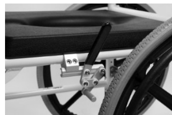
Pic. 4: Mounting of brakes to the frame
